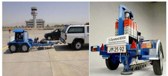
Heavy Weight Deflectometer (HWD) Falling Weight Deflectometer (FWD)
